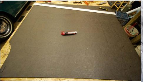
First he made a paper template for the two pieces. Then he glued four layers of roofing felt together for the outer section and glued two layers for the engine trapdoor. This allowed both surfaces to be even & flat. Finally he added a thin layer of "60 minute" roofing paper on top for smoothness.
