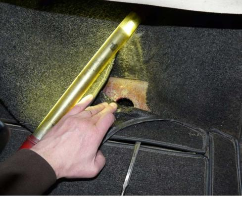
It was around midnight when Roland pulled-up the carpet behind the back seat in the area underneath the rear window shelf (above) and discovered two long bolts that had to be removed!Finally the body was apart from the chassis that same night (upper right). Philip was relieved to have solved that problem with the help of his friends and also happy to see onlyminor rust on the body to be repaired.
