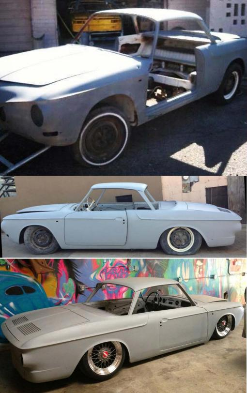
He quickly separated the body from the chassis. The body work done in nearby Tijuana Mexico at the reputable family-owned body shop of Don Jose. Within two months the pre-painted body was mated with the lowered chassis (previous page).Then it was sent to a good friend (Kekoat ARP Fabrication) for the air bag installation in July.
