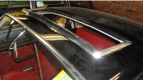
An original one (upper left) mounts to the front inner edge of the sunroof opening and is secured with screws into the roof metal. The outer edges of the deflector has a curved design. By comparison the repro deflectors has a more angled design (bottom). The repros are polished for a bright finish. Jurgen tested them on his own 1968 and fitted the felt seal over the deflector to make sure it seals properly.
