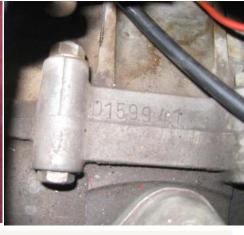
A numbers-matching T34, you can see the three VIN numbers (above). The chassis # plate is stamped under the rear seat, the body # plate is stamped into the aluminum plate inside the spare tire area, and the engine # is stamped into the engine case. Miguel's T34 has VIN # O 176 539 with original engine #O 159 941. Miguel plans to use it on an almost-daily basis from April to October except during the winter months that is usually cold and rainy in Europe.
