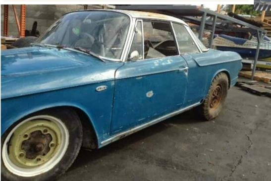
The body has some rust in the rocker panels & spare tire area. The chassis has rust in the rear floor area & in the battery area. The interior is destroyed, the dash pads are cracked, and the body has been mostly stripped. It does have its rocker trims, rear scripts, seats, & gauges.
