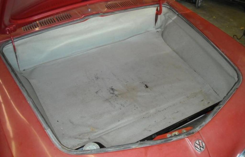
In October the exterior was coated in a thick layer of dust and nothing had been cleaned or detailed in many years. The engine was original & matching and featured the short black coil, rectangular air cleaner decal, anti-kink oil breather hose, and the early-style fuel pump. The only visible rust was along the edge of the inner spare tire well seam (below) which could easily be halted & touched-up.
