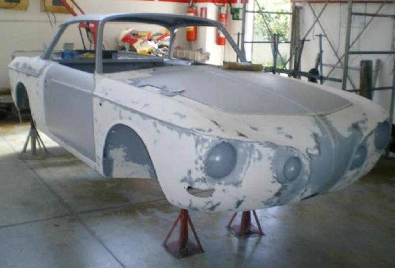
I began immediately to remove all possible parts of the car and quickly realized it was more and more in serious condition. I first sandblasted the entire body to see exactly what metal work would be needed. Shortly after that I began struggling with the engine and finally restored it, changing piston cylinders, heads, bearings etc. now a 1600cc with single carburetor. Recently I replaced the original muffler with an exhaust from ISP West.
