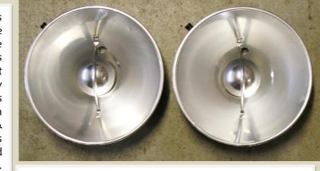
Once reassembled you can really see the difference. The "before" and "after" photo below shows what a difference the chrome spray paint makes. This process takes a couple hours and costs about \$20 total. For those on a budget that want a quick fix it's a good option vs spending \$150-200 or more.
