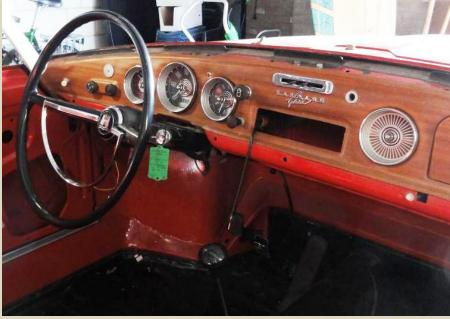
The instrument panel has been mostly reassembled with the exception of the dash pads & radio. The angled ignition switch is a quick indicator of a 1968 model year body which was mounted to the 1967 chassis. And if you look closely you can see the tiny dash warning light for the heated rear window. Below: the fresh electric sunroof headliner looks nice & tight. Nice work, Marc!
