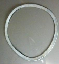
This is an original fog light to body seal. Made from a soft foam rubber, it's a simple flat design on both sides. And it seems so easy to reproduce too.
