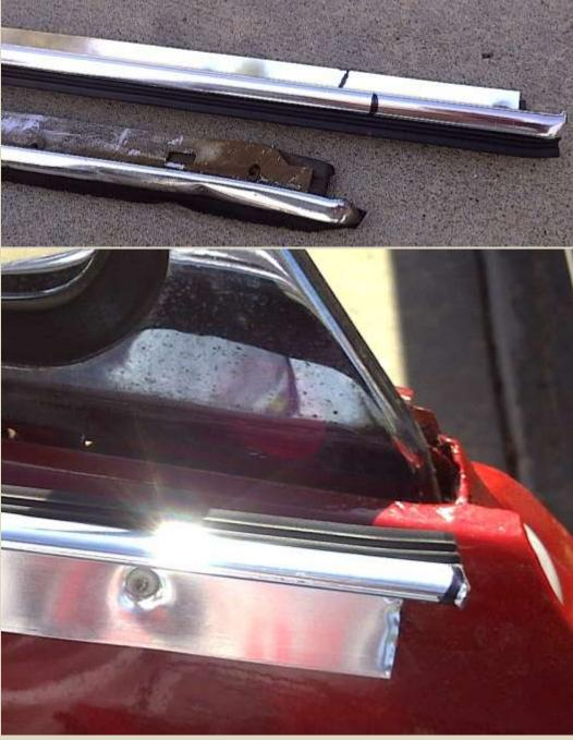
The next step is to mark the new window scrapers for trimming. The new ones are longer than the T34 ones (above top), but it's easy to mark the leading-edge to be cut & the metal is easily cut with tin snips. Once cut you should bend-down the cut edge like the original end looked. It's easier than it sounds ...
