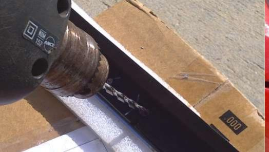
Once trimmed, the scraper can be fitted into the door top for marking the three mounting holes in the door. Mark the hole positions onto the new window scraper & drill holes into the scraper metal (above). The scraper can then be installed with the three sheetmetal screws with ease to look like new once again. I've found that sometimes the holes get enlarged and the original screws are too small to tightly fit the new scraper, so I've used larger screws for a nice secure fit.
