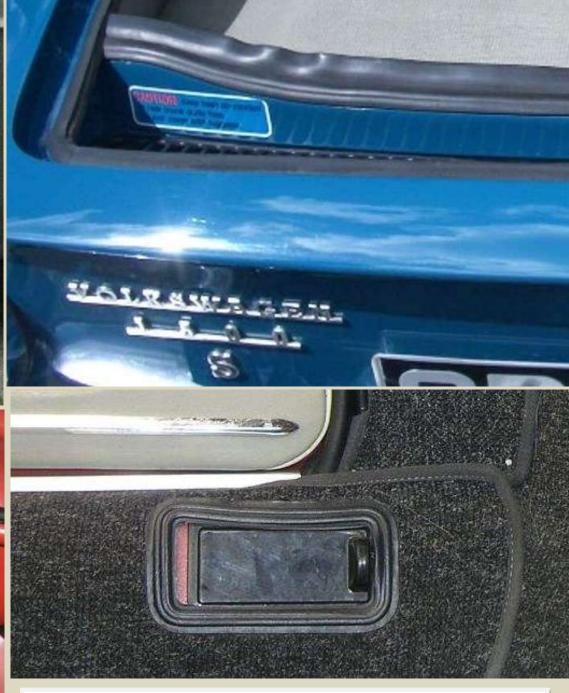
It was the last year for: painted hub cap VW logos, vertical jack storage position, amber gauge needles, push-button dash control unit, the plastic front heater sliders (above), the light-gray two-toned shift knob, the rear compartment decal warning about keeping loose items in the air duct (top photo), and aluminum rear view mirror stem.
