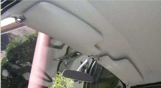
1966 T34s were a hybrid, sharing parts from the early & late models. They had the bumpy vinyl, rounded base & rounded chrome arm of the early style but they had the driver's side pocket & passenger's side vanity mirror. Pics of a restored set are on the right. Rounded bases & arms with pocket/mirror.
