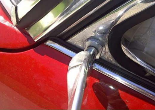
You can see once the scrapers are installed that the trimmed front edge looks original despite being trimmed. The rear edge should just slightly overlap the door window seal.
