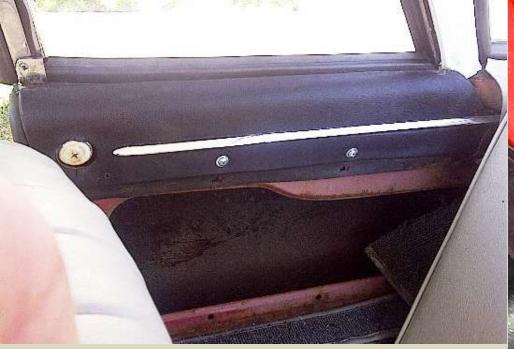
Since the rear quarter pads (above) were a bit rusty underneath (and no replacements available), I was forced to mount them over the quarter window seal lip and secure them with long sheetmetal screws into the metal body. Sometimes you have to make-do and once better ones are located the problem will be solved. T34 restorations are never really completed 100% ...
