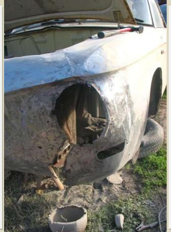
But with the windows in I decided to tackle the front end again. I pounded-out as much metal as possible but I had split a poorly welded seem under the driver's side headlight (right pic). Luckily I found a mig welder in my price range the next week. After the paint was applied the T34 was really coming along as I headed into 2011.
