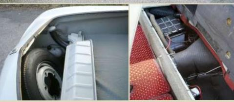
Unique to 1962 several parts are painted to match the body color: engine trapdoor metal, spare tire cover, and seat frames. The engine trapdoor cover is a solid Silver-Beige material without the Auf/Zu text or arrows. Other unique 1962 features include the solid ivory shift knob, two-piece fresh air vent trims, front seat backrest release mechanism at the top of the seats, Lemmeritz beauty trim rings that hug the outer edge of the rims, "cat's eye" side mirror, and large oil dipstick head.
