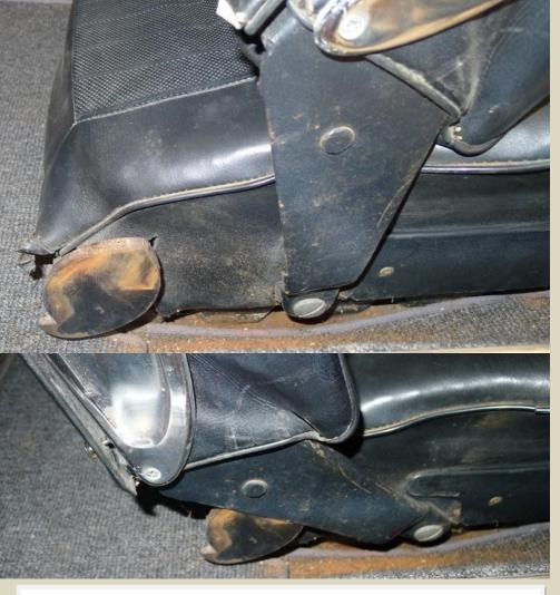
The **1966 style** (above) saw the elimination of all seat locking components and the seat was able to be folded forward at any time. Obviously this was not safe while driving and was quickly discontinued for the late-model design.
