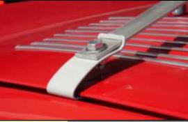
The roof racks have six feet that have black tubing to protect the gutter from scratches. There are two quick-release clamps that mount securely under the aluminum roof gutter trim. Leather straps are an optional item to give it a period-correct look. The slim profile allows air flow into electric sunroof opening also.
