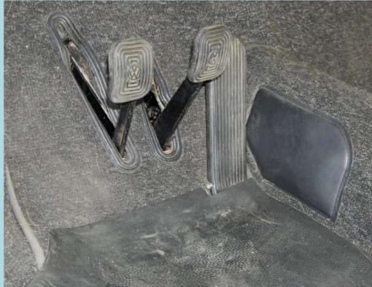
A closer inspection of an original 1968 carpet kit (above) reveals the edges are bound in vinyl, not cloth & Velcro pieces are sewn into the front heater pieces to mate with the floor mats so everything stays in-plate. He also noticed the back-side of these pieces were coated with some sort of moisture proofing that makes them much heavier than the earlier non-coated carpets.
