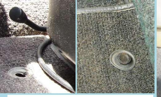
Carpeted floor mats were fitted beginning in 1966 and included the carpet trims for the floorpan buttons (above in 1967: two per mat for front & rear) and the heel & side foot pads (below: in 1967). Right lower pic: rubber floor mats fitted in 1962-65.
