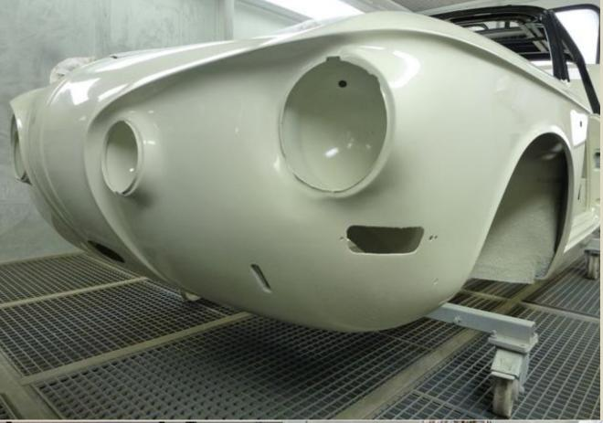
The Carblast painter picked up the T34 in November 2011 for the painting process. It was Cathodic dipped by January 2012 and small holes in the front fenders were discovered. He repaired the holes and spent 120 hours to prepare the body for paint. By July the body was painted Lotus White (L282) and the roof Black (L41), and the entire T34 was clear-coated. The painter will deliver the finished 1966 back to Michael in August.
