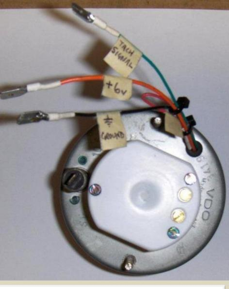
The wiring that was connected to the terminal 1 of the coil is now connected with the green wire on the tach.
