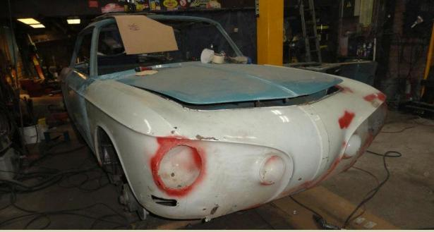
The original rusty headlight metal sections (above) were too bad so they'd welded a new clip into place. This is a common rust area in T34s. With no repro headlight metal panels available, this 1968 will
