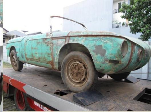
The chassis appears to be solid & original. The strange metal added to the rear window sheetmetal is unique, obviously added as some sort of reinforcement area for the folding top. The original 5-lug rims & brakes are still on the front but the rear has 4-lug rims so there's a bit of sorting-out to be done there.
