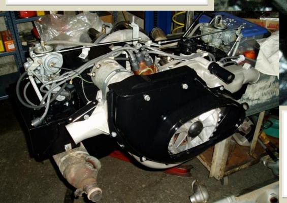
Many months later the engine came back. Seeing as it was the original, numbers matching motor I wanted a very original rebuild. Paul the builder reworked the original early single port heads, knurled the dome top pistons, reamed the original cylinders, and did some other magic that is normally reserved for the Formula V engines he builds. As a result the rebuilt motor made 74 sea-level horsepower on his dyno. I placed this new motor under the car in the back of the garage.
