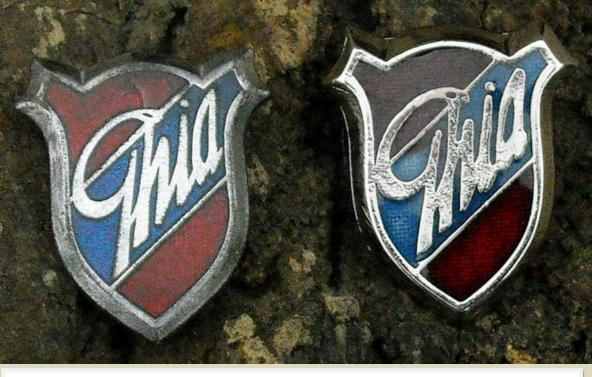
The repro shield is easily identified from the back by the patterned surface. From the front side it's not so easy ... but isn't that the point? This original 50 year old shield (above left) is well worn. Below: a view from inside the panel.
