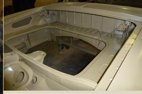
These photos were taken after the triple-series of chemical dipping to remove the paint, rust, & apply the anti-rust coating of primer paint. You can see the original tin, used to join the metal panels at the Karmann factory, has been removed, so these seams will be finished-off next. This dipping process is essential to be confident all of the rust has been removed forever.
