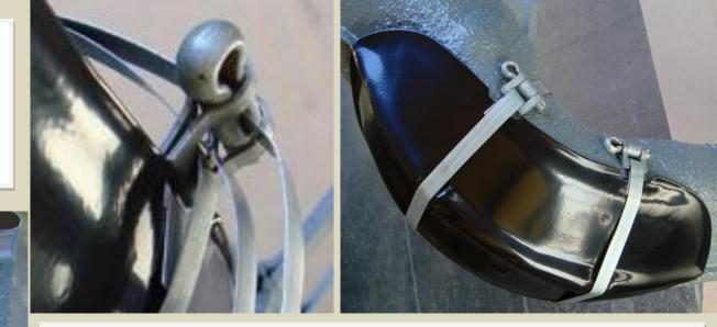
Position the shield & straps loosely. Originally VW had the clamps on the inboard sides. The strap wraps around the heat exchanger once, threads through the rectangular hole on the clamp, then wraps around a second time and threads through the cotter key. Pull in the slack and then trim off some of the excess strapping. Then tighten the key with a screwdriver a half-turn at a time, stopping to adjust the strap and reposition as necessary as you go. Turned out very nice!
