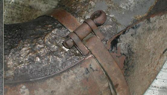
I did some research on substitutes for the coating and settled on Lizard Skin (www.lizardskin.com) ceramic insulation. It's not cheap but it has properties that make it a good choice for the job: good heat & sound insulation, withstands temperatures to 500°F, water based & non-toxic. I applied it with a brush over ISP West's ceramic coating, recreating the original texture, and then gave it several coats of engine enamel.
