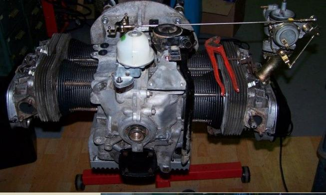
I also had all of the non-chrome metal galvanized parts including the door window regulators, screws, & bolts. Black powder-coating was applied to the engine sheet metal and spare tire carrier. The fuel tank was rusty so it was de-rusted first and then coated with a plastic solution inside. The engine was rebuilt & reassembled. lt's nice to see these old parts new once again!"
