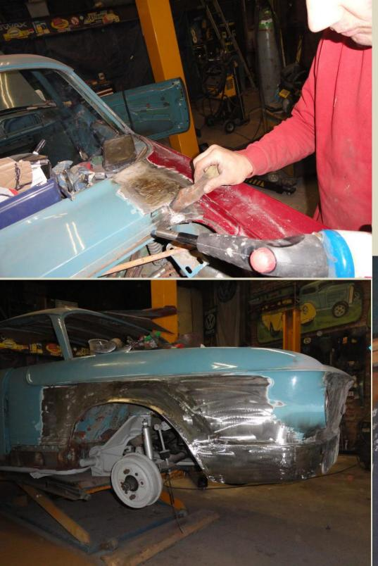
You can see the left-rear fender metalwork in bare-metal form after the wheel arch was welded into place and a hand-formed lower rear corner section was created by Jurgen. The lower-left photo shows Chris drilling-out the weld spots along the left rocker panel area.
